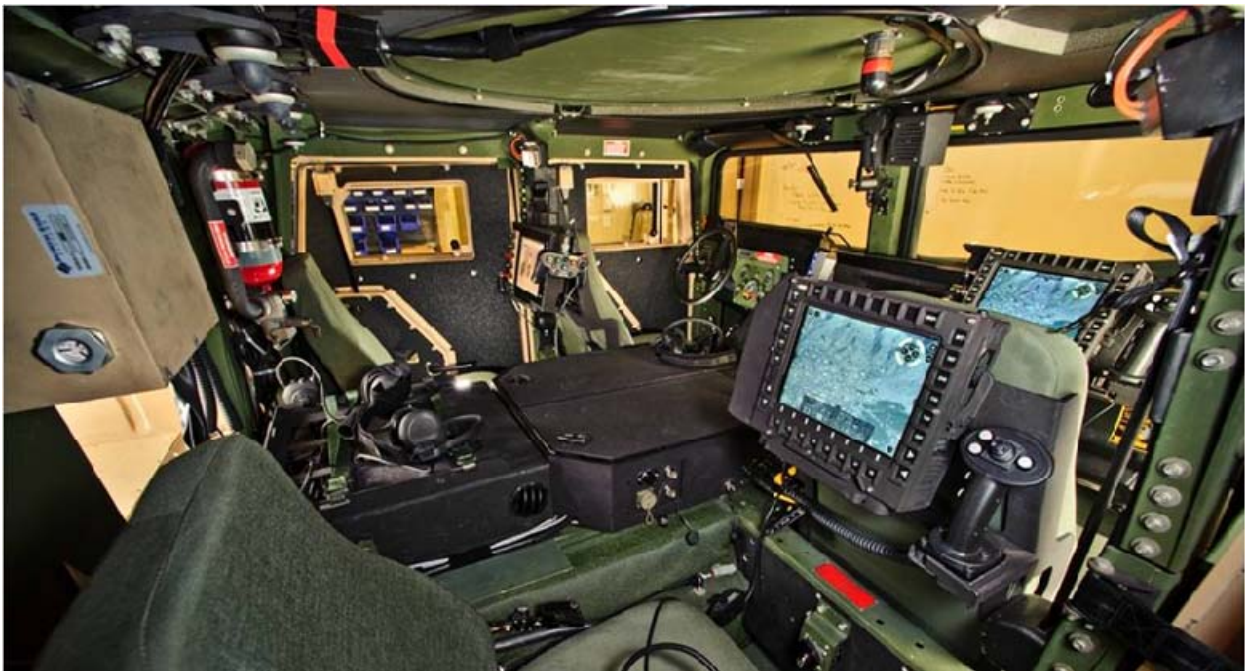
Figure 3: Multi-function smart displays reduce the amount of hardware that must be installed in a vehicle
