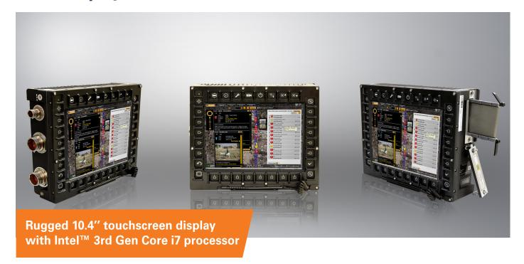
The SD8010's 3rd Gen Intel™ Core-i7 processor provides cutting-edge computing capabilities suitable for the most demanding in-vehicle applications.
